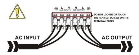
Do not loosen or touch the rear set screws on the terminal block.
