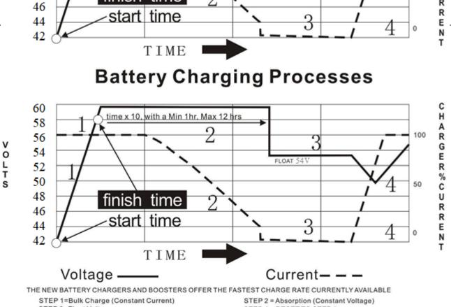
STEP 3=Float Voltage STEP 4 = RESET TO STEP 1
