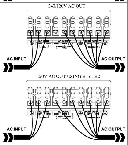
\*\*The *pump output* will only be used when a pump struggles to operate smoothly when connected to the primary AC output of the inverter. This output has an additional inline transformer for added inductance and is less efficient than the primary AC output terminal block. Do not use this output if the pump operates normally when connected to the primary AC output. Batteries will discharge faster when connected to the pump output.
