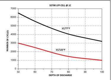
At high temperatures, the SEI film decomposes, cracks, or dissolves, resulting in continuous consumption of lithium ions and rapid decline in capacity.
