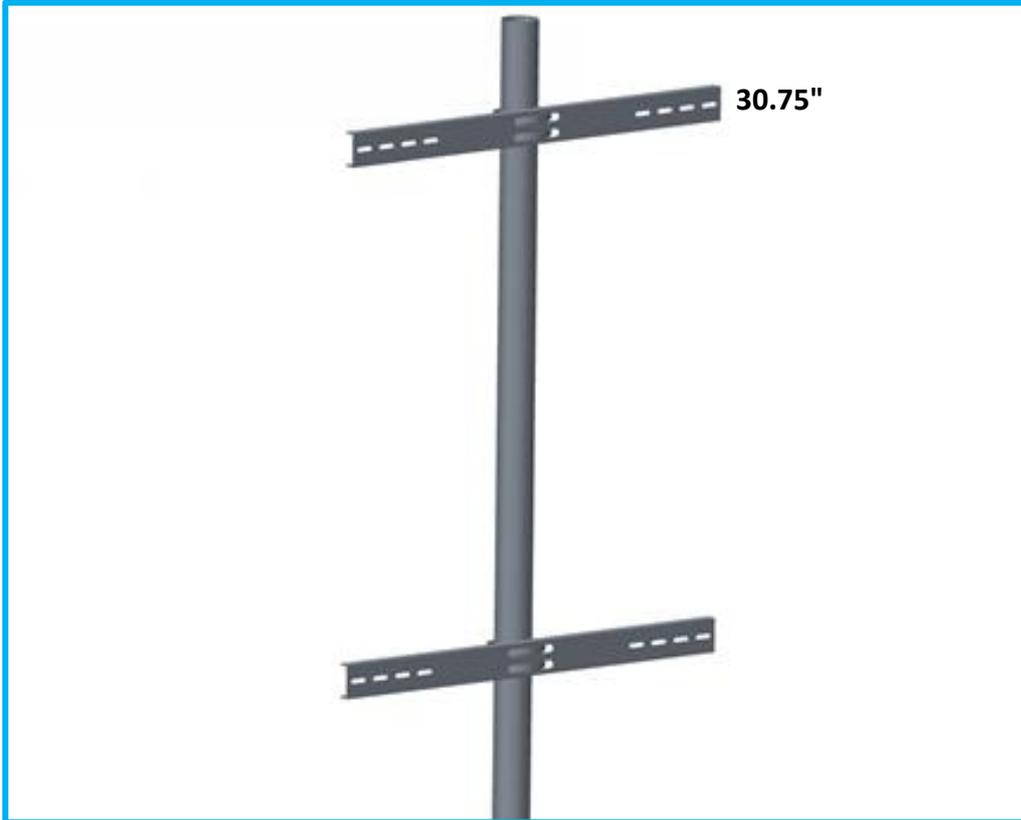
2. Secure upright brackets and support brackets to pole brackets using angle brackets and bolts. Once secure, set angle by sliding the loose hose clamp up or down and tighten.
