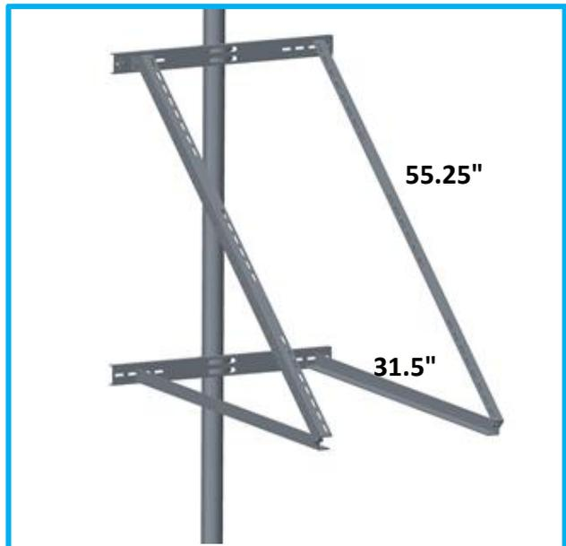
**3. Place the solar panels horizontally on the upright brackets and attach using bolts (panels should have pre-drilled holes on the back).**
