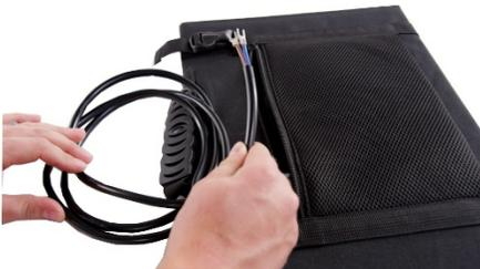
2. The wires connect to a charge controller via the spade lug on the end. Some charge controllers may connect via bare wire. If this is the case, simply cut off the spade lugs and slide bare wire into the controller.
