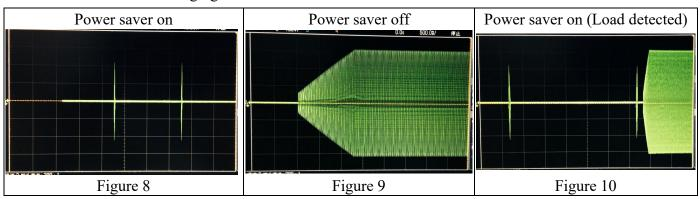
Note: The minimum power of a load to take inverter out of sleep mode (Power Saver On) is 50 Watts. For split phase models, the power threshold of sleep mode is 50W between Hot1 and Neutral and 200W between Hot 1 and Hot 2. There is no load detection between Hot2 and Neutral.
